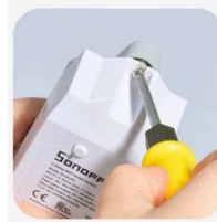
Install the switch on the tray with screws
