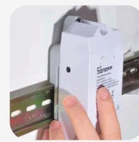
Then mount it on the DIN rail until secure
